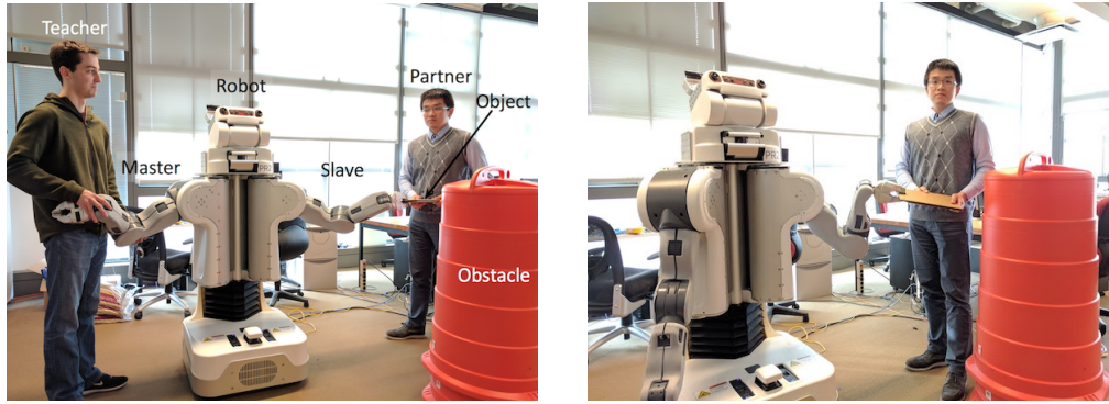
(a) The teacher guides the robot to manipulate an object with the partner.
