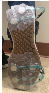
(b) Event switches on a shoe sole.
