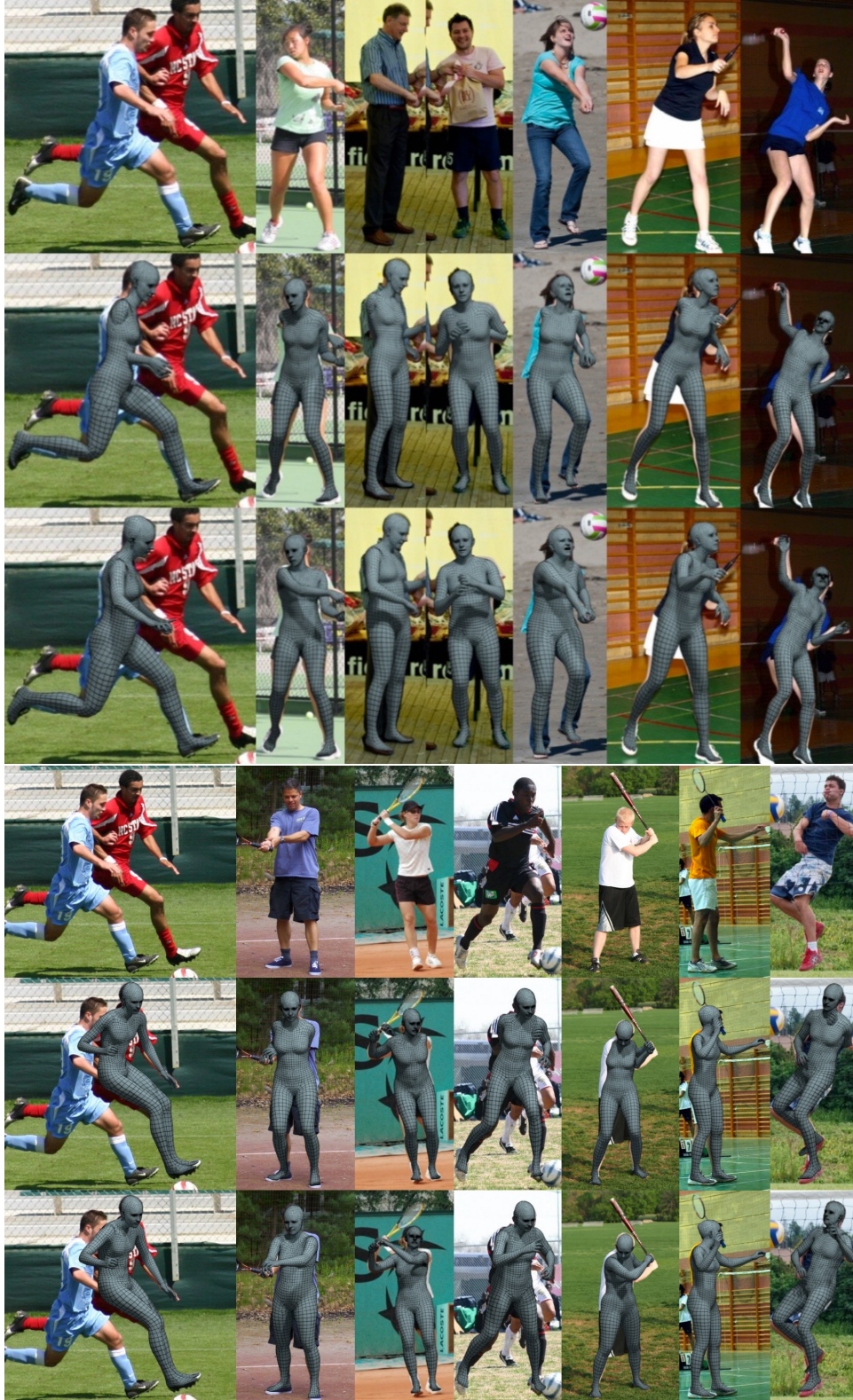
Figure A.15. Results of SMPLify-X fitting for the LSP dataset. For each group of images we compare two body priors; the top row shows a reference RGB image, the bottom row shows results of SMPLify with VPoser, while the middle row shows results for which VPoser is replaced with the GMM body pose prior of SMPLify [5]. To eliminate factors of variation, for this comparison we use the gender neutral SMPL-X model.
